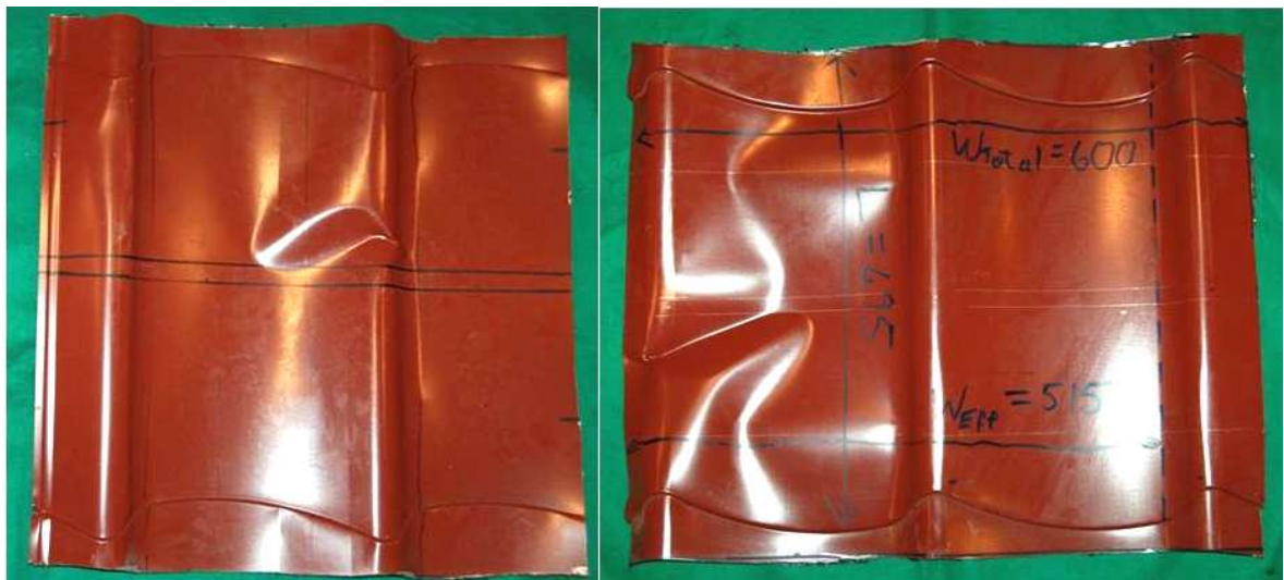
Figure 2: Samples removed from sheeting, shown after testing. Note the localized plastic deformation, and absence of any visible fracture..
